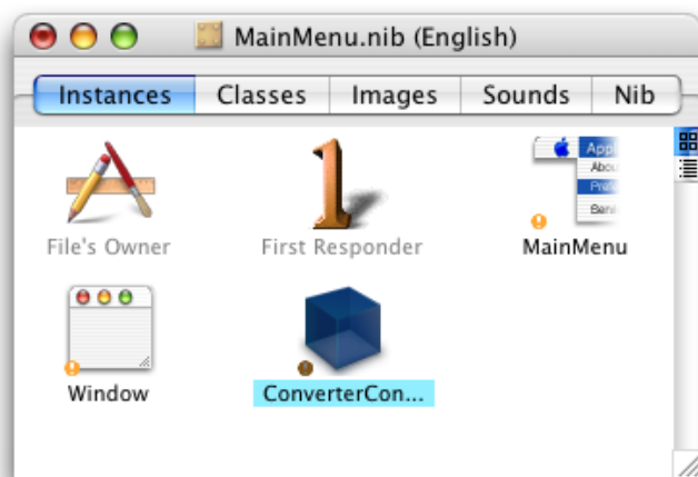
Figure 2-21 A newly instantiated ConverterController instance
