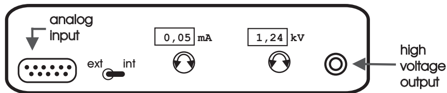
Figure 6: Front view of the high voltage power supply used to drive the Pockels cell.
