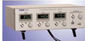
Figure 3.7: Picture of the Piezo Controller MDT693A used to control offset voltage of the piezo.
