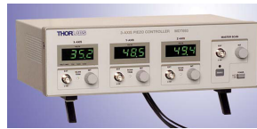
Figure 4.4: Picture of the Piezo Controller MDT693A used to control offset voltage of the piezo.
