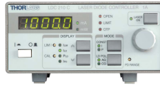
Figure 4.3: Picture of the Laser Diode Controller LDC202C used to stabilize and control the current fed to the laser diode.
