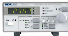
Figure 3.8: Picture of the Thermoelectric Temperature Controller TED200 used to stabilize the temperature of the laser diode.
